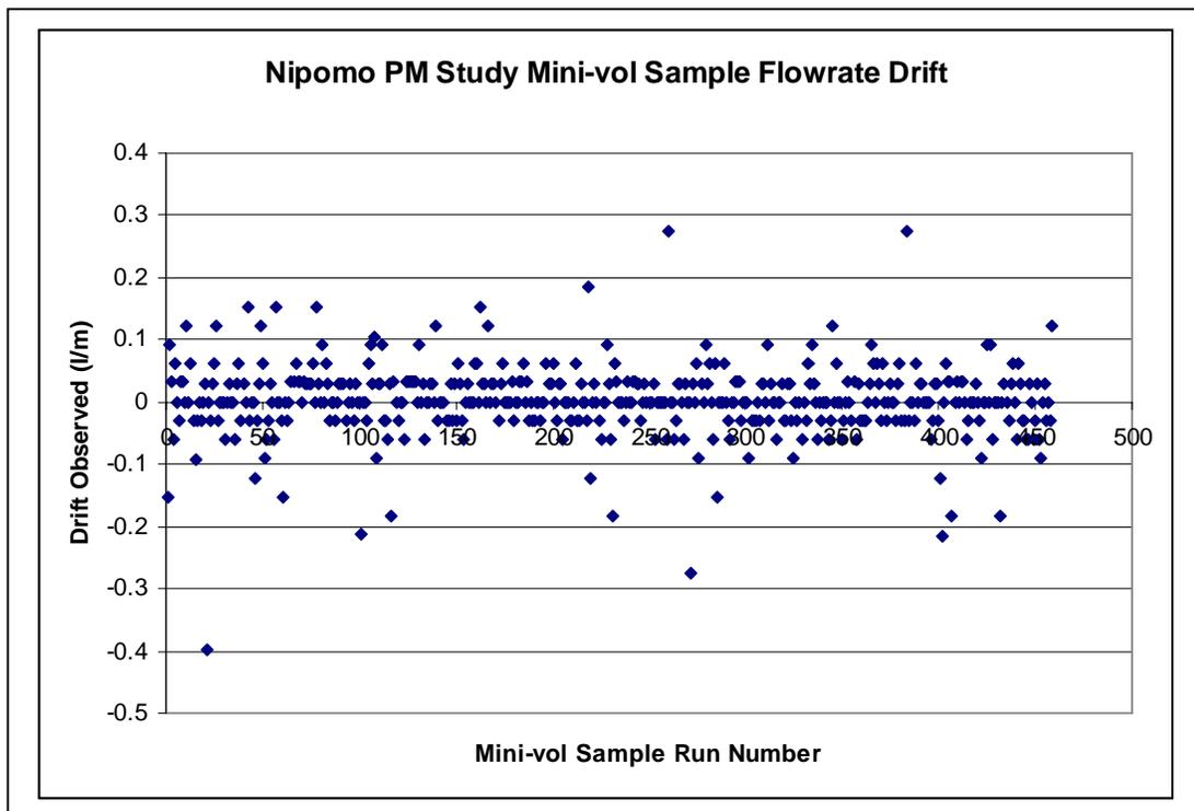
**Figure A-4. PM2.5 Sampler Flowrate Drift**
