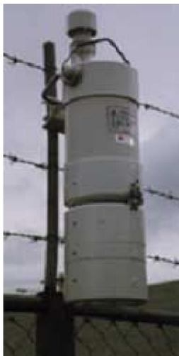
**Figure 2. PM2.5 Mini-Vol Sample Example**
