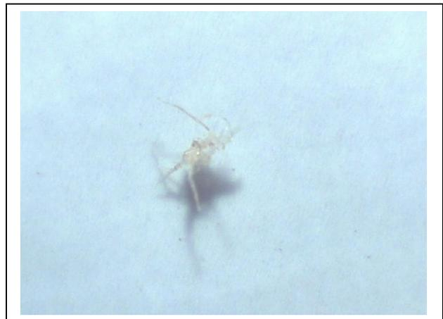
Filter jcpft261 with evidence of contamination (X60)
